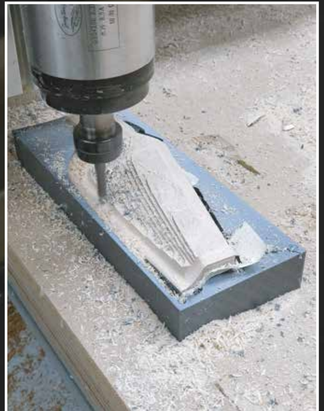
Our second revised headstock design was CNC machined from a single piece of Maple wood.
